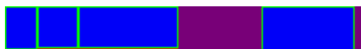
Figure 2. In this visual representation of a cache page, surfaces are outlined in green, red areas represent wasted space and purple represents available space.
